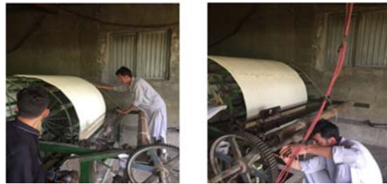
Figure 7: Arhat (Wheel) used for Warping Threads on a Warp Beam
